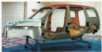
nents are joined together through a unique adhesive bonding system which eliminates mechanical fasteners. The bonding system contributes to the structural strength of the space frame and speeds the production process. Ashland Chemical supplies the adhesive.
